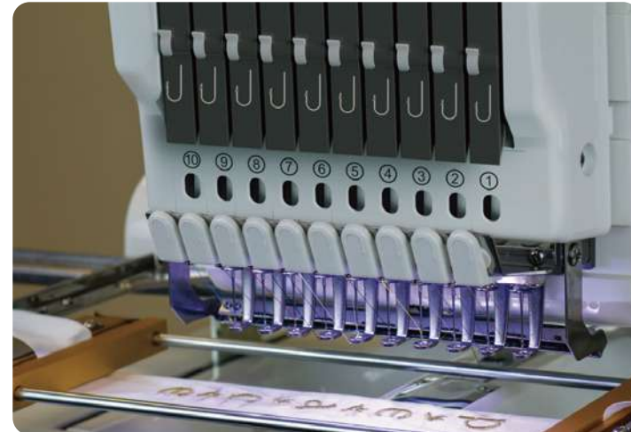
Belt Hoop (BH-3) With an 8-inch x 4-inch embroidery area, the belt hoop allows ample room for embroidery on belts and straps.
