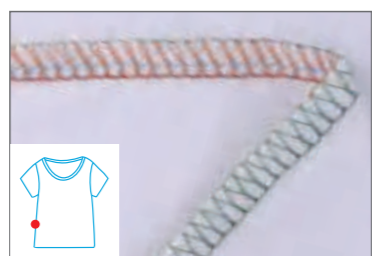
Four Threads Basic Stitch C6-4-M03/333/KS
