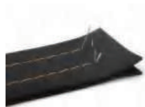
Condense stitch lock, short thread remaining
