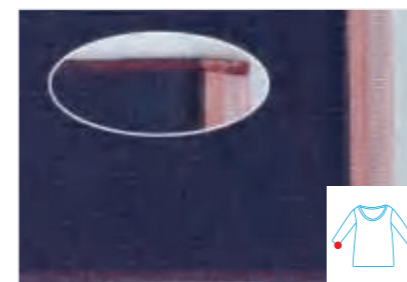
Three threads back latching stitch
