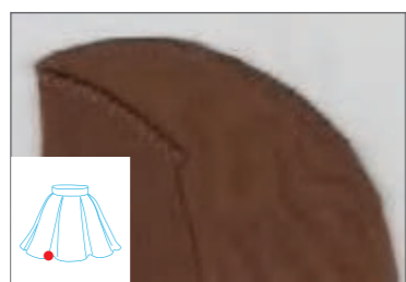
Three Threads Condense Seaming C6-3-32R2/223/KS
