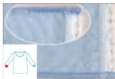
Four Threads Pneumatic BackLatch Seaming C6-4-83/323/BK
