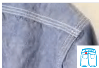
Triple needle chain stitch
