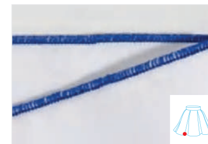
Three threads baby overlock stitch
