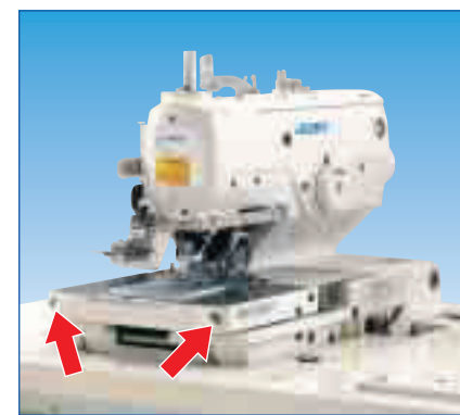
Material opening amount adjusting screw MEB-3200SS
