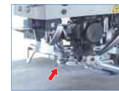
Needle thread clamp device
