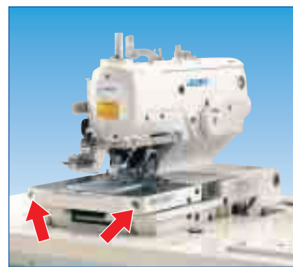
Material opening amount adjusting screw MEB-3200SS
