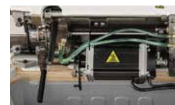
Stepping motor drive for the thread trimmer and auto-lifter
