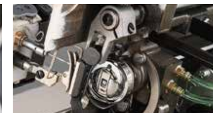
Lower side of the thread-trimming knife
