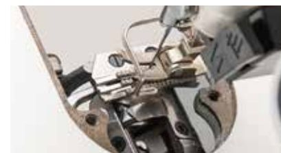
Upper side of the thread-trimming knife
